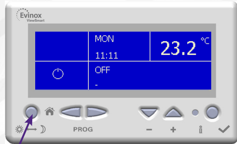
1. From the Home Screen - Press the Home button to view the Main Menu.
